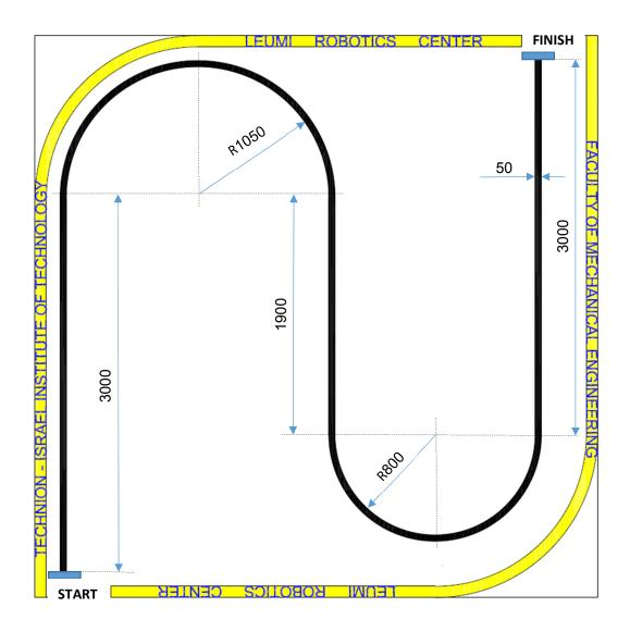
The car must reproduce the specified route as accurately as possible on the site without lines.
