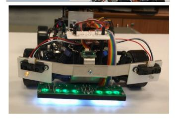
The Robotraffic - 2018 participants should add to car 9 LEDs. Three (3) LEDs (in front of the car) indicate and repeat the traffic light's signals (simultaneously). Two (2) LEDs in the car front and two (2) LEDs in the back are for indicating of turns. Two (2) LEDs in the car back are for the stop indication. Please contact Roman (Skype: sroman777) for the additional information.
